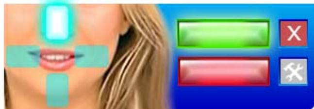
This error is due to a connection issue between PSPIX and the computer (network connection with PSPIX not configured or incorrect, Ethernet cable disconnected, PSPIX OFF).
